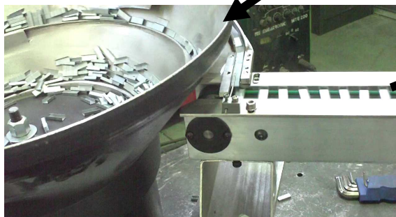
Staples strips adjustment with vibrator
